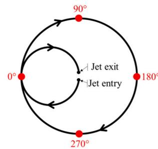
**Fig. 2.** Cutting path strategy used in this study. The four orientations correspond to the roughness measurements.
