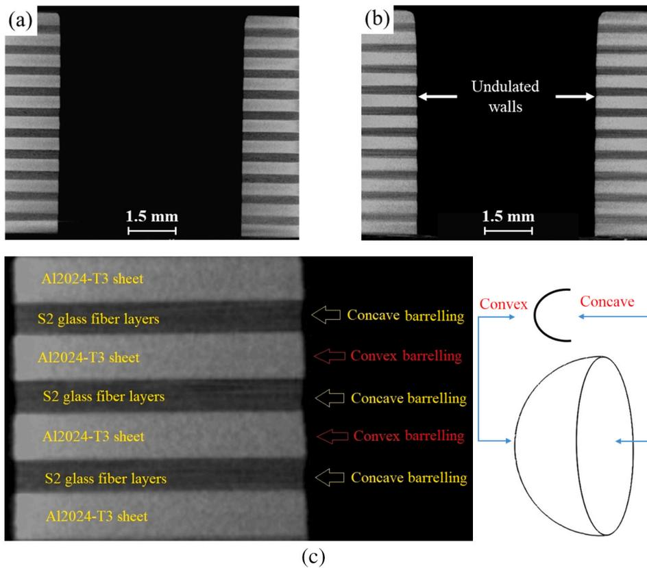
Fig. 5. CT scans of holes drilled by AWJ with  $P = 124$  MPa,  $AFR = 360$  g/min, (a)  $SoD = 2.5$  mm and (b)  $SoD = 5.0$  mm (c) Convex and concave barrelling phenomenon in aluminium sheets and glass fibre layers.
