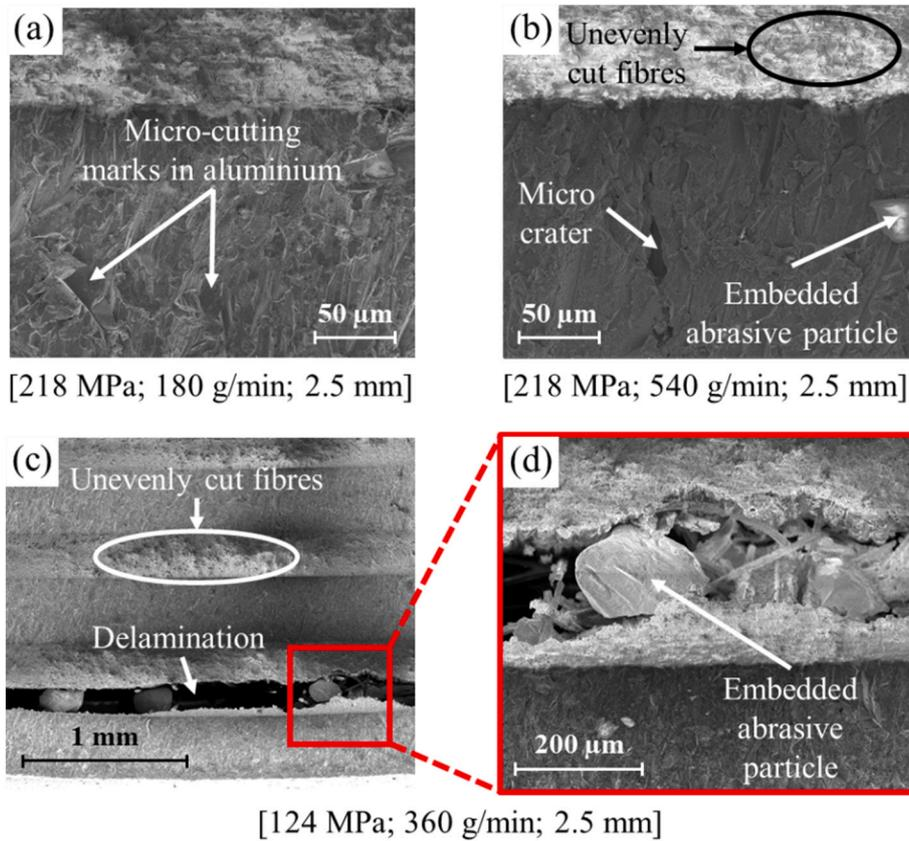
Fig. 8. SEM pictures showing the defects induced by AWJ drilling on GLARE with: (a) micro-cutting marks, (b) micro-craters and embedded particles in aluminium, (c, d) unevenly cut fibres in GFRP and delamination with embedded abrasive particles at the interface.
