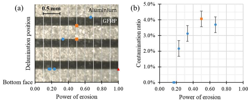
Fig. 11. Position of the delaminated plies (a) and contamination ratio (b) as a function of the “power of erosion”.
