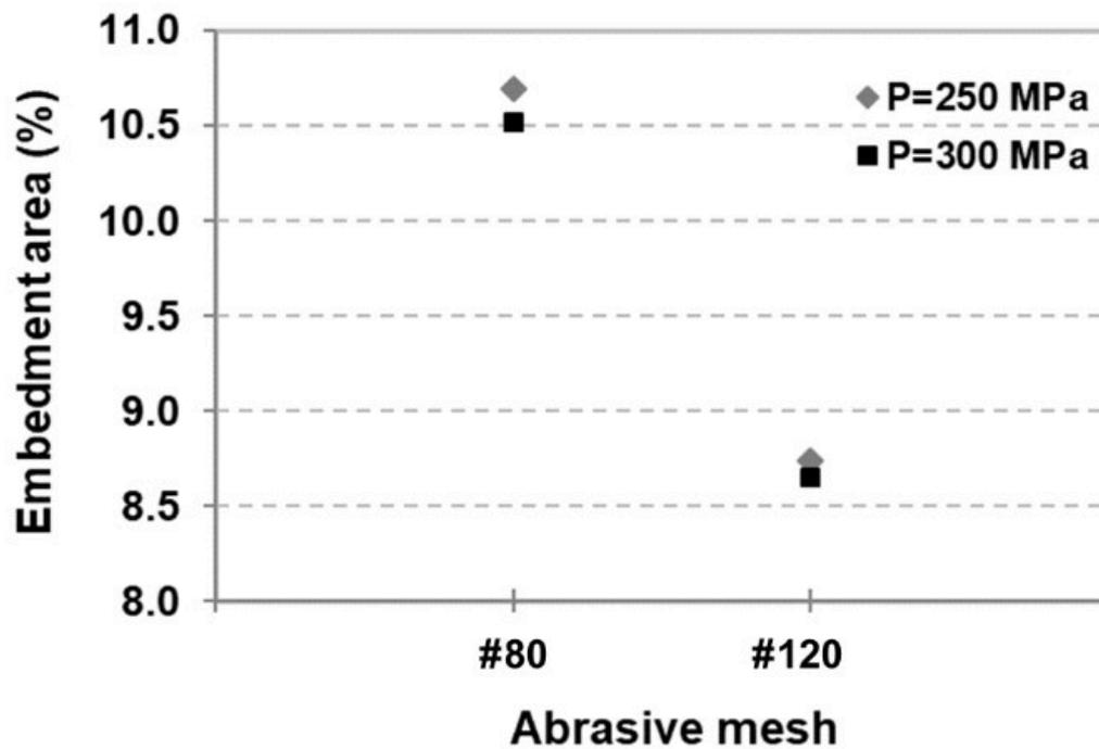
Fig. 7. Influence of grit size and pressure on abrasive embedment area.
