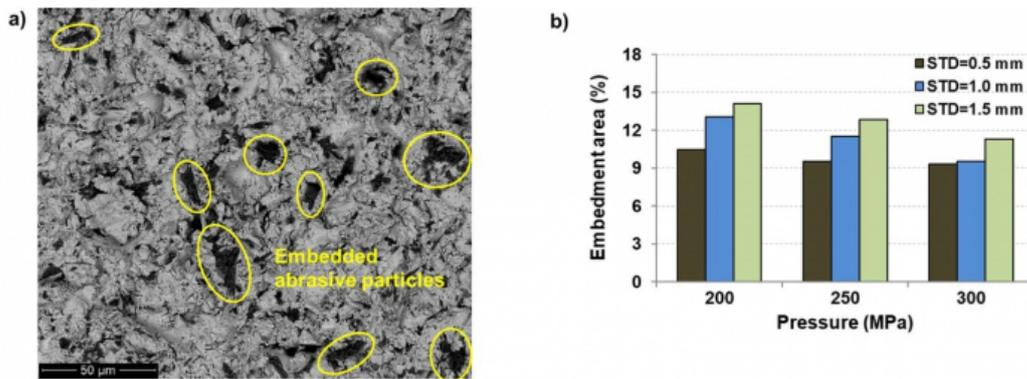
Fig. 3. (a) SEM micrograph of third pocket of the specimen milled at  $P = 250 \text{ MPa}$ ,  $f = 1.5 \text{ m/min}$  and  $STD = 1 \text{ mm}$ ; (b) Percentage of abrasive embedment area in function of the jet pressure and step-over distance.
