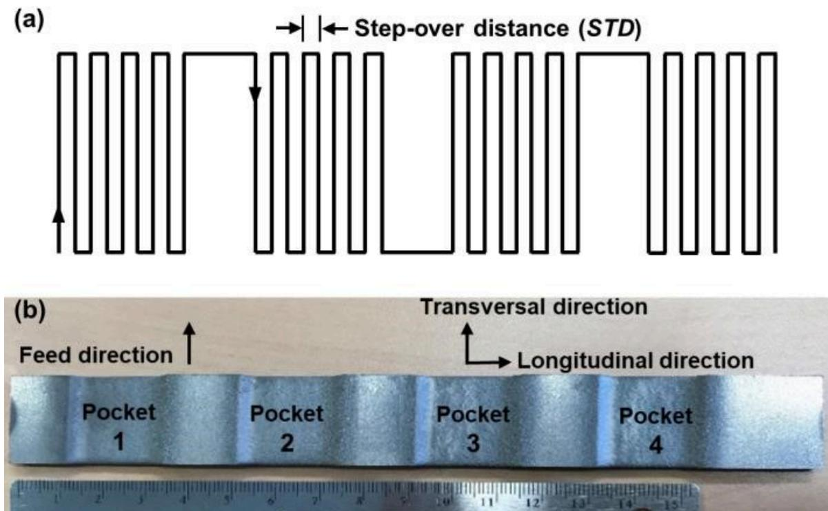
Fig. 1. (a) Tool path; (b) Sample machined at  $P = 250 \text{ MPa}$ ,  $f = 1 \text{ m/min}$  and  $STD = 0.5 \text{ mm}$ .
