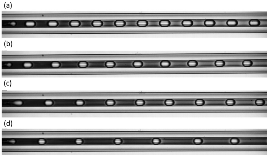
Fig. 12. Generation of a two-phase segmented flow of \text{CO}_2 and \text{BPB}/\text{H}_2\text{O} for 10 MPa and 303 K where \dot{V}_{\text{CO}_2} = 82.5 \mu\text{L}\cdot\text{min}^{-1} : (a) \dot{V}_{\text{H}_2\text{O}} = 110 \mu\text{L}\cdot\text{min}^{-1} , (b) \dot{V}_{\text{H}_2\text{O}} = 150 \mu\text{L}\cdot\text{min}^{-1} , (c) \dot{V}_{\text{H}_2\text{O}} = 200 \mu\text{L}\cdot\text{min}^{-1} and (d) \dot{V}_{\text{H}_2\text{O}} = 300 \mu\text{L}\cdot\text{min}^{-1} .
