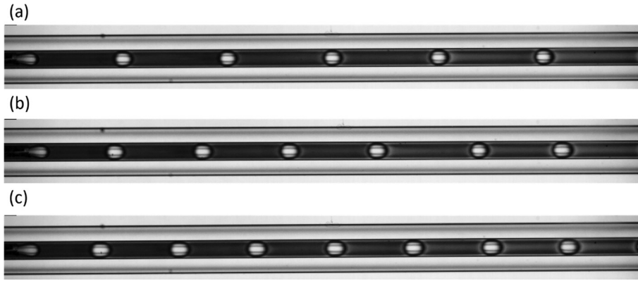
Fig. 11. Generation of a two-phase segmented flow of \text{CO}_2 and \text{BPB}/\text{H}_2\text{O} for 10 MPa and 303 K where \dot{V}_{\text{H}_2\text{O}} = 350 \mu\text{L}\cdot\text{min}^{-1} : (a) \dot{V}_{\text{CO}_2} = 76.6 \mu\text{L}\cdot\text{min}^{-1} , (b) \dot{V}_{\text{CO}_2} = 94.2 \mu\text{L}\cdot\text{min}^{-1} and (c) \dot{V}_{\text{CO}_2} = 111.9 \mu\text{L}\cdot\text{min}^{-1} .
