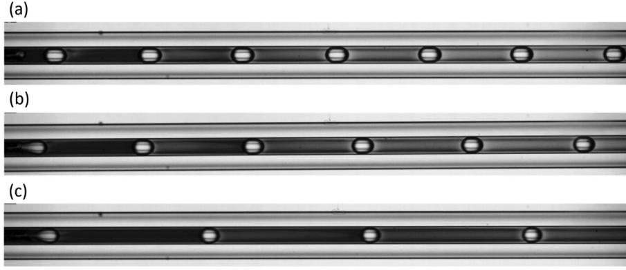
Fig. 10. Generation of a two-phase segmented flow of \text{CO}_2 and \text{BPB}/\text{H}_2\text{O} for 10 MPa and 303 K where \dot{V}_{\text{CO}_2} = 58.9 \mu\text{L}\cdot\text{min}^{-1} : (a) \dot{V}_{\text{H}_2\text{O}} = 150 \mu\text{L}\cdot\text{min}^{-1} , (b) \dot{V}_{\text{H}_2\text{O}} = 200 \mu\text{L}\cdot\text{min}^{-1} and (c) \dot{V}_{\text{H}_2\text{O}} = 300 \mu\text{L}\cdot\text{min}^{-1} .
