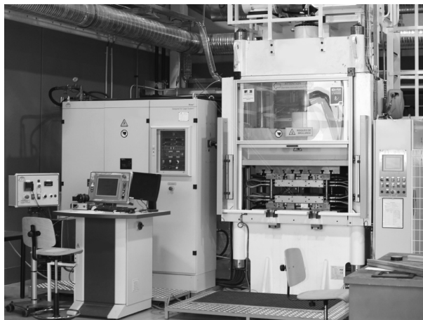
Figure 8 – Thermo-compression pilot plant with induction-heated mould
