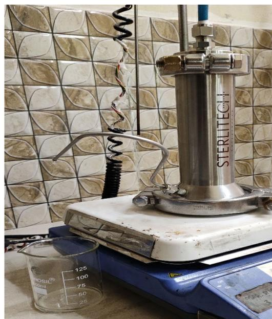
Fig. 1 Dead end filtration technique using Sterlitech model HP4750 stirred cell
