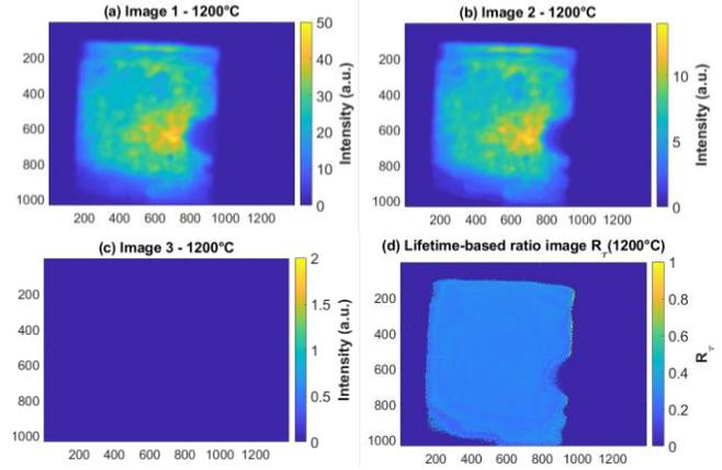
Figure 8: (a)-(c) Example of a series of fluorescence intensity images captured by the camera CCD (at 694 nm) and (d) corresponding lifetime-based ratio  $R_\tau$  map obtained on a 15x20 mm<sup>2</sup> coated sample after 10 min exposure at 1200°C.
