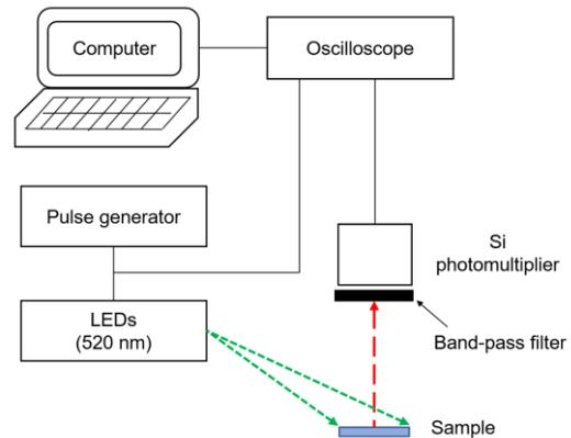
Figure 4: Experimental setup for luminescence lifetime measurements.
