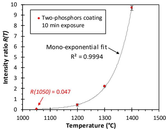
Figure 3: Calibration curve  $R(T)$  vs. Temperature for 10 min exposure of the bi-phosphor coatings between 1050°C and 1400°C. Dashed line corresponds to the fit of the experimental data points with a mono-exponential model.
