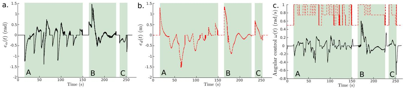
Fig. 5: a. Angular error (in rad) – b. Distance error (in meters) – c. Angular velocity and controller used. For the controller plot : GtG controller = 0.5;  $\omega_B$  controller = 1 and  $\omega_A$  controller = 0.75.
