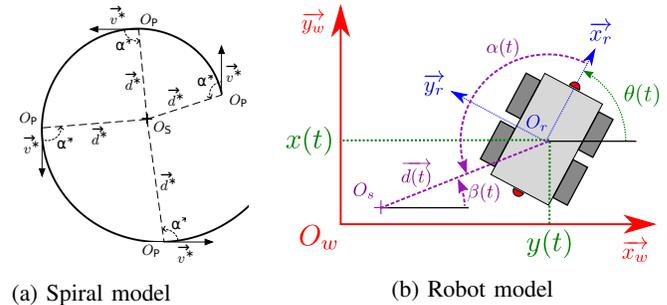
Fig. 1: Spiral and robot modelling
