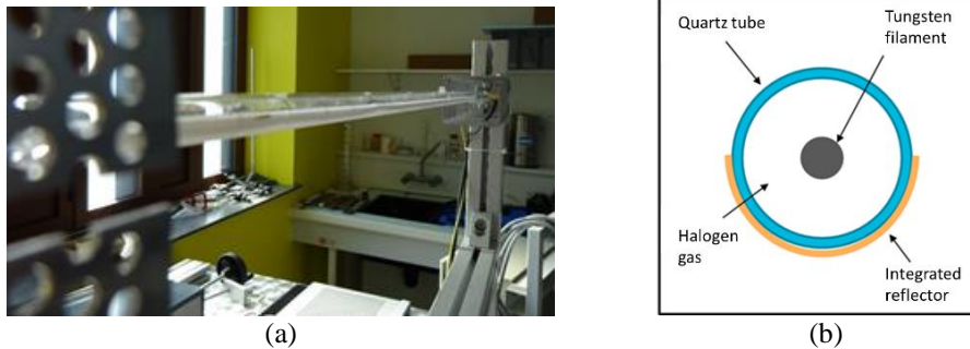
FIGURE 1., (a) Infrared halogen lamp with integrated reflector,(b) schematization
