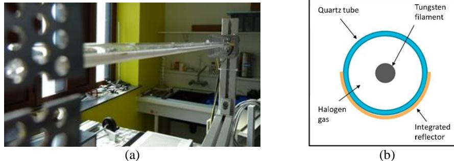
**FIGURE 1.**, (a) Infrared halogen lamp with integrated reflector,(b) schematization
