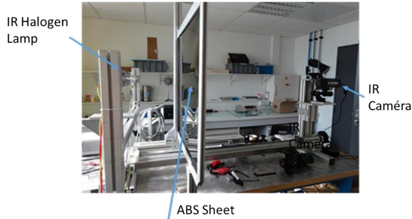
**FIGURE 2.** Experimental set-up
