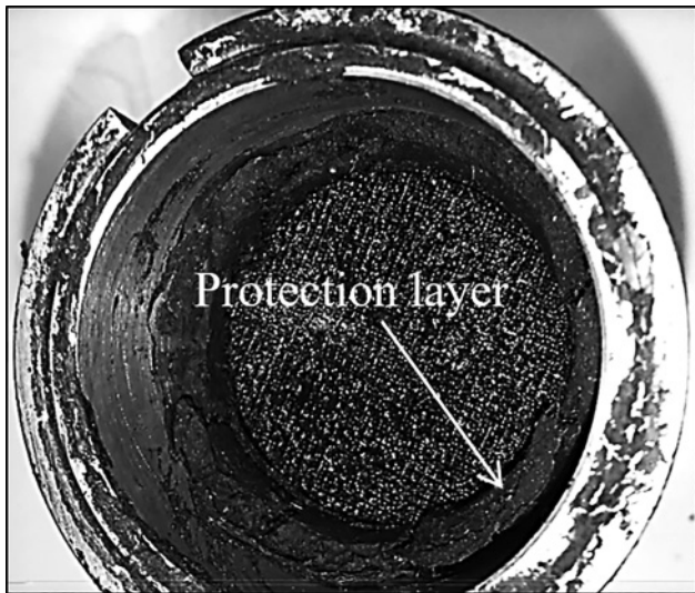
Figure 6 | Picture of the sludge after 3 hours of experiment at 80 °C for 20 wt.% TS sludge.
