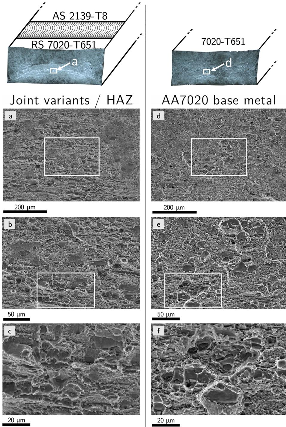
**Fig. 12.** SEM fracture surface features at several magnifications. (a, b, c) welded joint (condition BW03): mixed mode fracture composed of dimples initiating from small intermetallic particles and transgranular fracture from elongated grains, (d, e, f) AA7020 base metal – dimples close to each other and only elongated grain features.
