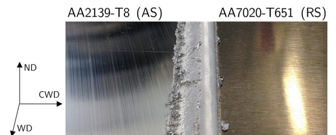
Fig. 6. Top view of weld surface with defect formation due to inappropriate welding parameters.
