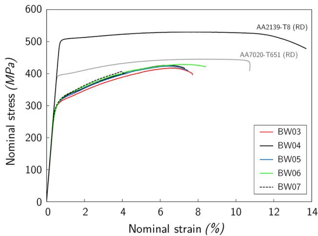
**Fig. 10.** Stress-strain curves for base metals and the five welding conditions. For each condition, one curve among the 3 performed was chosen (For interpretation of the references to color in this figure legend, the reader is referred to the web version of this article).
