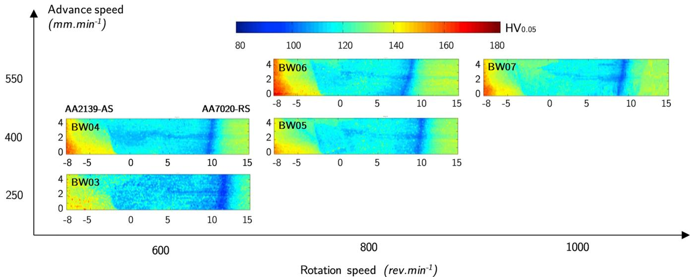
**Fig. 9.** Microhardness maps ( $\text{HV}_{0.05}$ ) for the five conditions inside the process window.
