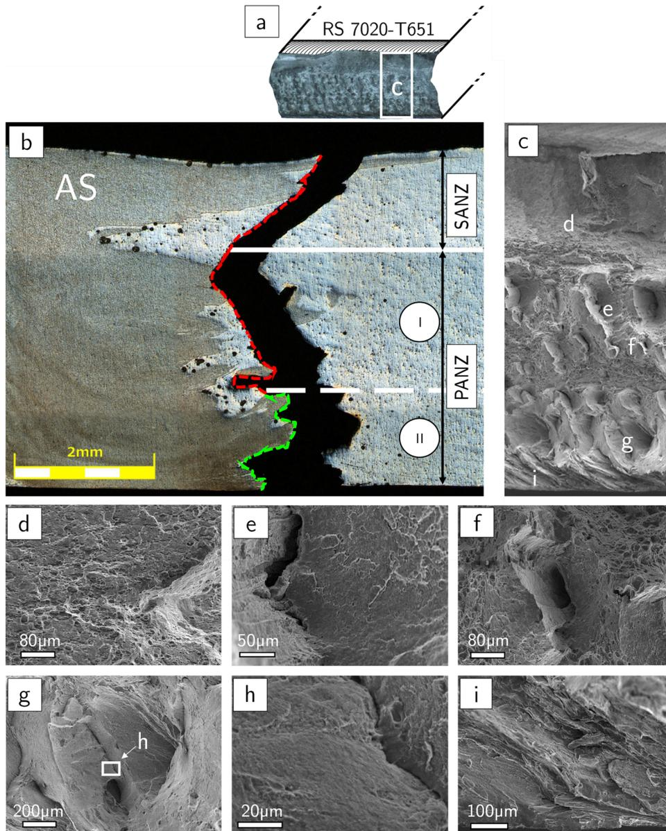
**Fig. 13.** Fracture on a BW07 sample failed in nugget: (a) Position of area “(c)”, (b) Cross weld section with green dotted line for the interfacial fracture and red dotted line for the non-interfacial fracture, (c) Fracture surface revealing homogeneous SANZ and periodic PANZ. In PANZ, two regions can be found according to surface morphology (zones I and II), (d, e, f, g and h) Zoom of various areas on the fracture surface in (c).
