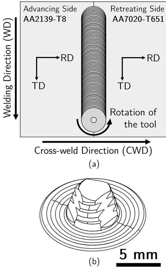
Fig. 1. (a) FSW setup and material orientation for the dissimilar welding trials (RD: rolling direction, TD: transverse direction); (b) 5 mm FSW tool with Triflat<sup>™</sup> pin and scrolled shoulder used for the welding trials.
