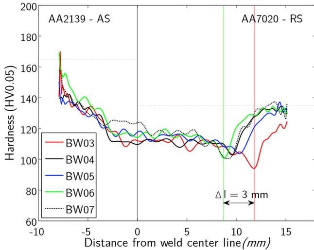
**Fig. 8.** Microhardness profiles at mid-thickness for the five welding conditions. Horizontal dot-lines show base material hardness while vertical green and red lines are the two extreme positions of the MHR function of the welding parameters. (For interpretation of the references to color in this figure legend, the reader is referred to the web version of this article).
