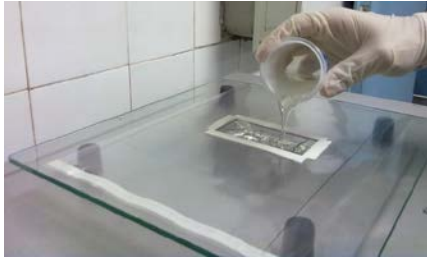
Figure 2. Deposition of the photoresist (step 1 of the micro-manufacturing process).
