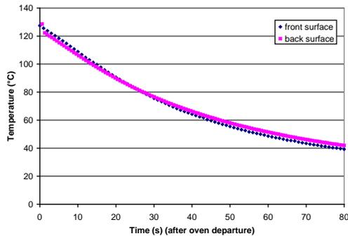
Figure 6- Cooling of the HPP sheet
