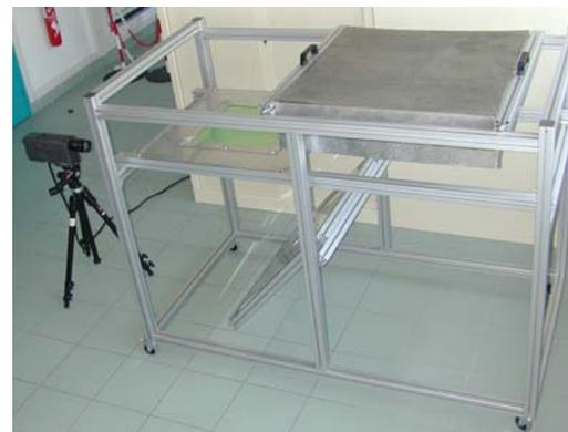
Figure 5 - Experimental infrared heating set-up
