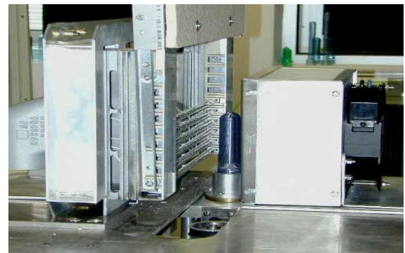
Fig. 5 Experimental infrared Oven Set-up
