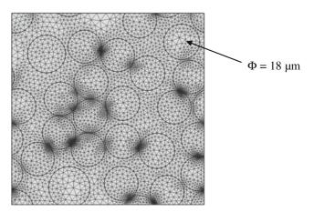
Fig. 6 Typical mesh used for the computations
