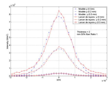
Fig. 12 Intensity distribution of the laser beam for different values of y: 0 mm, 0.2 mm and 0.5 mm (Rectangular shape)
