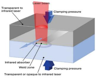
Fig. 1 Laser welding system [1]
