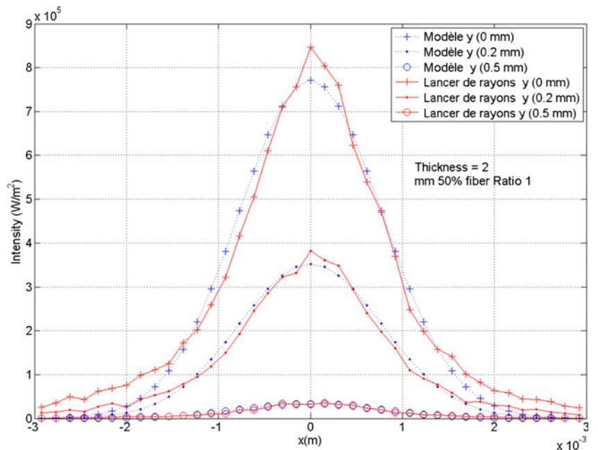
**Fig. 12** Intensity distribution of the laser beam for different values of  $y$ : 0 mm, 0.2 mm and 0.5 mm (Rectangular shape)
