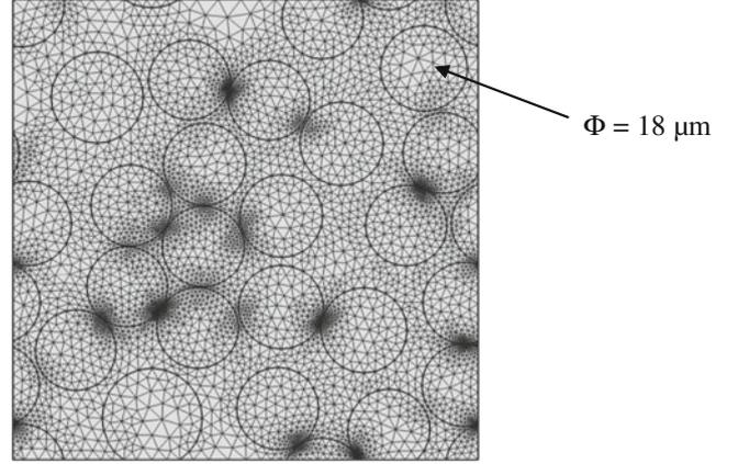
Fig. 6 Typical mesh used for the computations
