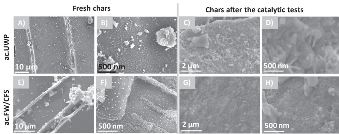
Fig. 4. SEM images of the activated chars ac.UWP and ac.FW/CFS before and after the ethylbenzene cracking tests at 650 °C.
