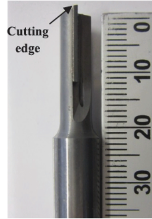
Fig. 2. PCD tool used with two straight flutes.
