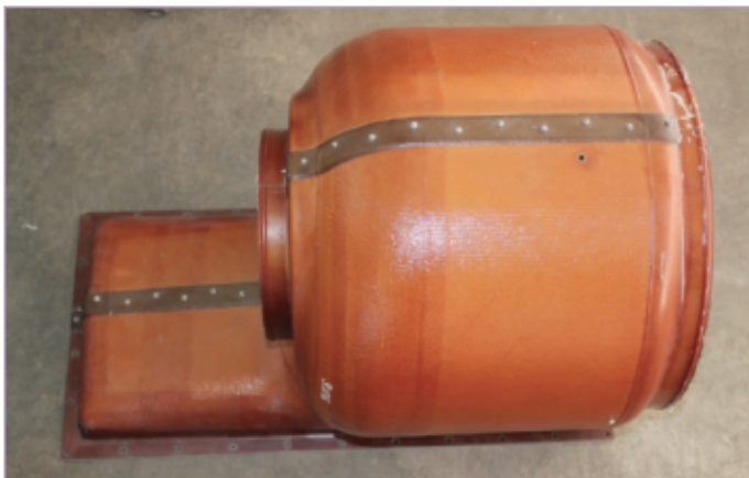
Fig. 1: Current design of the plenum, courtesy of Liebherr Aerospace
