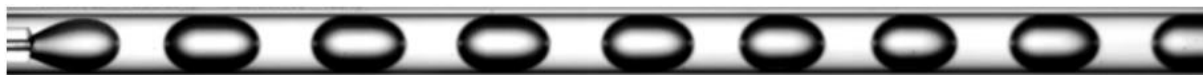
Figure IV. P = 20 MPa; T=308 K; V CO 2 = 0.02 mL.min -1 ; V H 2 O = 0.02 mL.min -1 in a 530 µm capillary.
