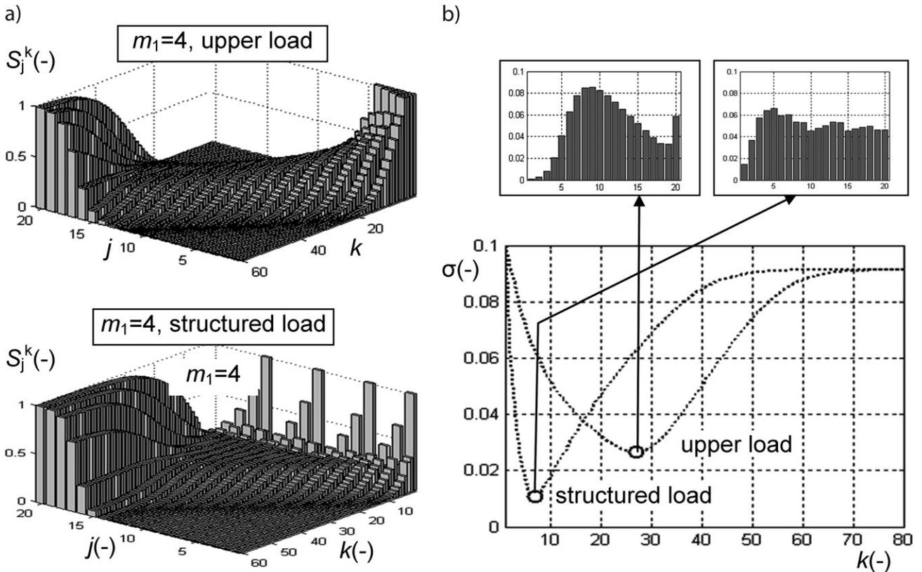
**Figure 3.** Comparison of mixing characteristics at the upper and structured load: (a) evolution of the key component distribution at different ways of loading; (b) mixing kinetics for different ways of loading (small windows above the graphs show the relative distribution of the key component at optimum mixing time).
