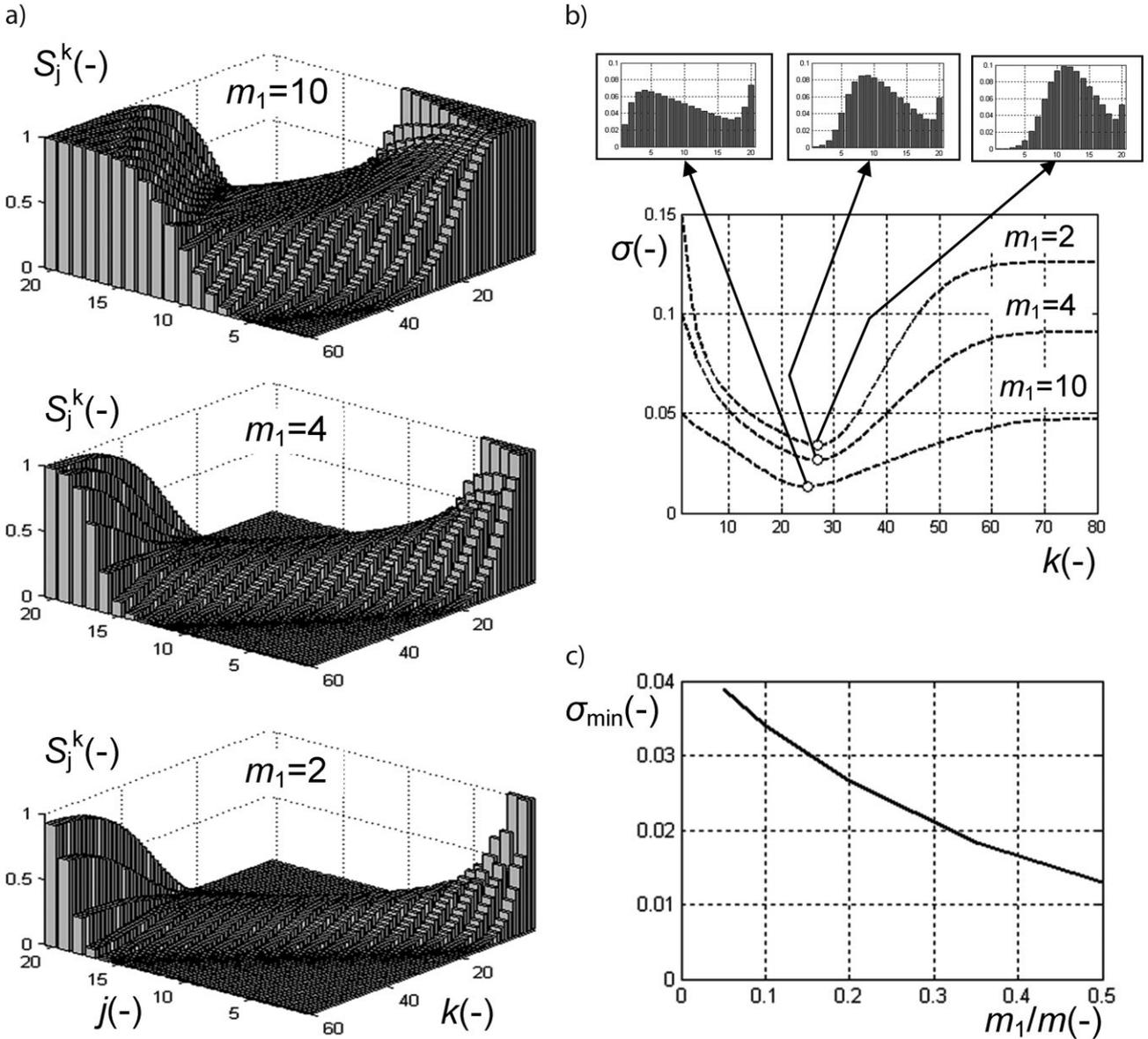
**Figure 2.** Influence of the key component amount on mixing characteristics: (a) evolution of the key component distribution at different amounts of the component; (b) mixing kinetics for different amounts of the key component (small windows above the graphs show the relative distribution of the key component at optimum mixing time); (c) influence of the key component amount on the minimum reachable non-homogeneity.
