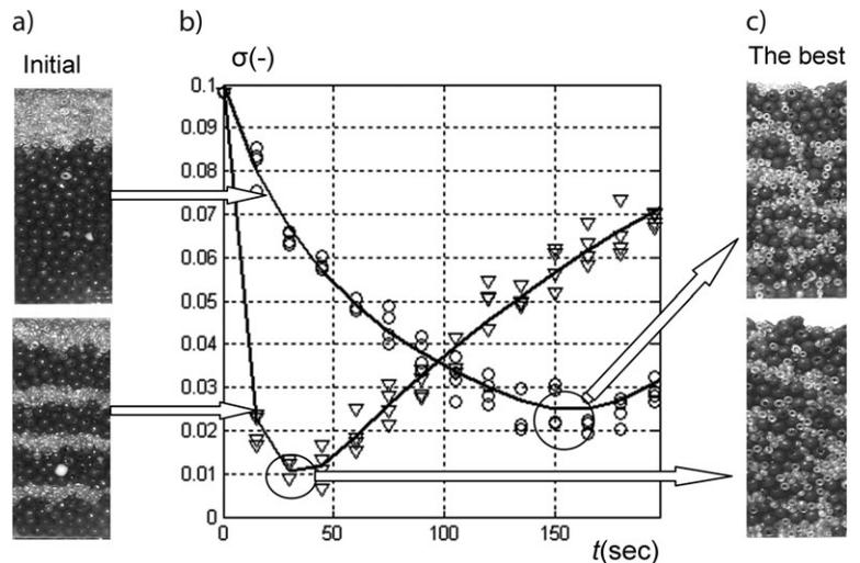
**Figure 5.** Experimental comparison of mixing kinetics for two ways of the key component loading: (a) photo of initial distribution; (b) experimental (points) and calculated (lines) mixing kinetics; (c) photo of the best distributions that can be reached.
