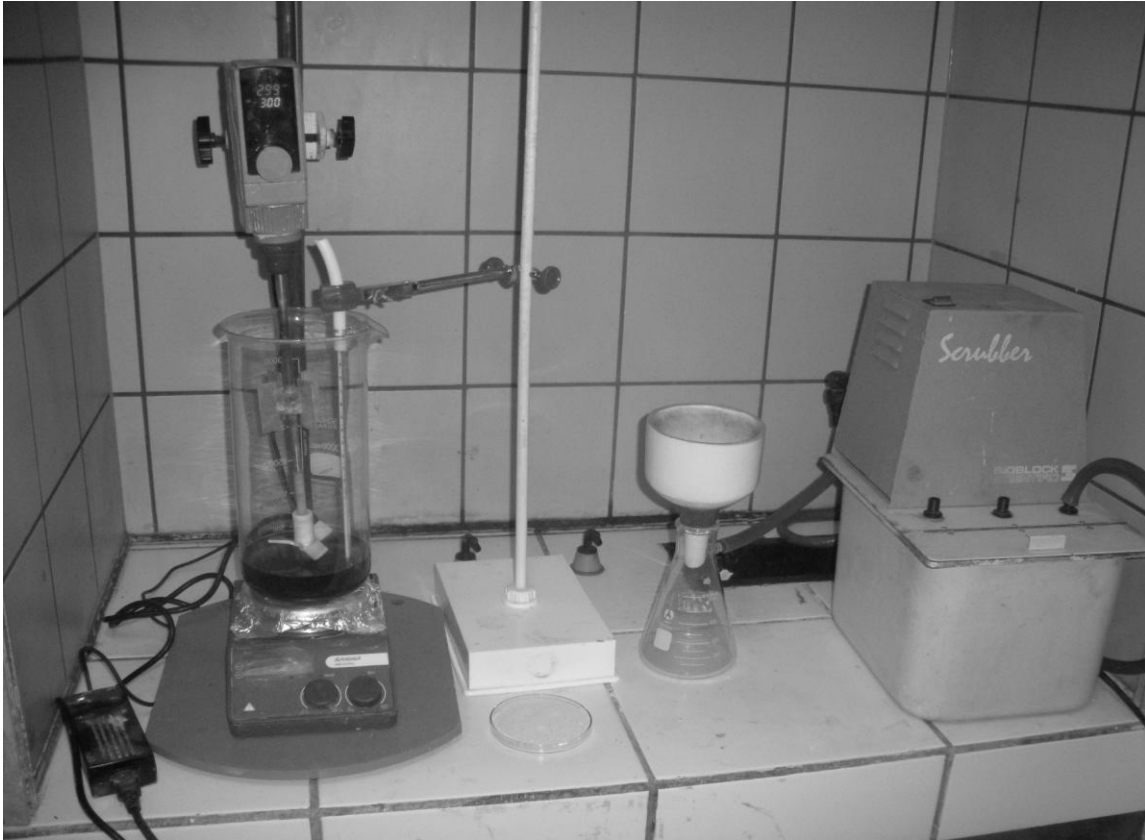
Figure 1. Experimental design of the attack of the phosphate by industrial phosphoric acid.
