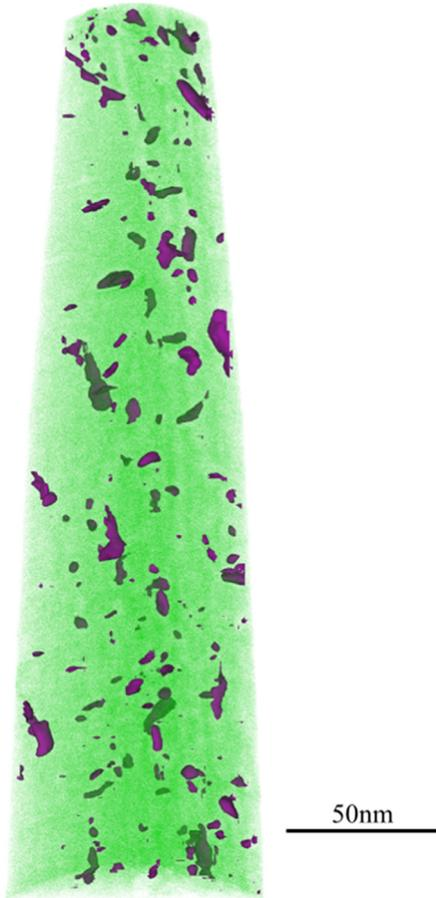
**Fig. 12.** Three-dimensional APT reconstruction of Ni atoms (green) of a sample tempered at 516 °C for 10 h. Carbides are represented as violet isoconcentration surfaces (total concentration of Mo and C is 36 at. pct). (For interpretation of the references to color in this figure legend, the reader is referred to the web version of this article.)
