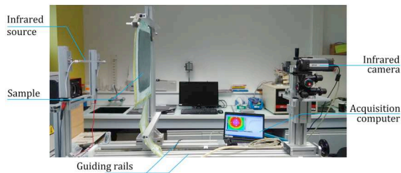
Fig. 2: Experimental 1 lamp heating test bench
