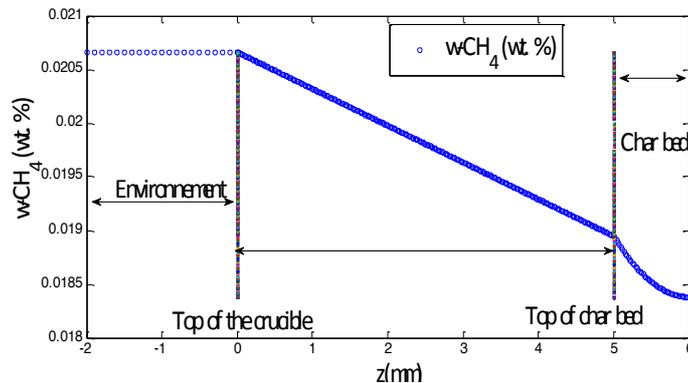
Methane concentration profile for the maximum reaction rate at  $900^\circ C$
