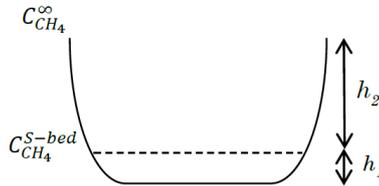
Fig. 1. Schematic representation of the TGA crucible
