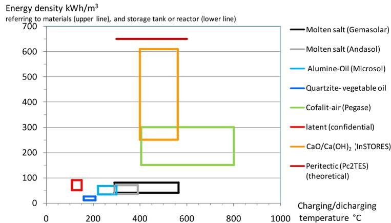
**Fig. 8.** Energy density of TES systems experimented in Fedele laboratories. Upper lines refer to the material volume. Lower lines refer to the tank or system volumes and are indicative values measured on non-optimized laboratory devices or prototypes. Only black and gray lines correspond to well-known commercial CSP plants.
