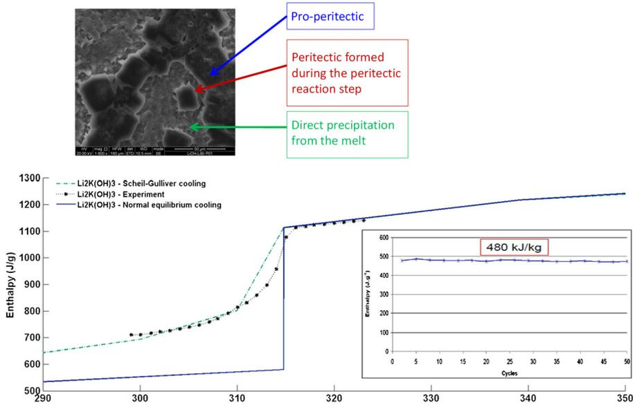
Fig. 7. Summary of the experimental results obtained for  $\text{Li}_2\text{K}(\text{OH})_3$ . Bottom: enthalpy-temperature curve (symbols: experimental points; continuous lines: theoretical calculations); insert: enthalpy change measured during successive cycles of heating and cooling. Top: SEM image of the final material.
