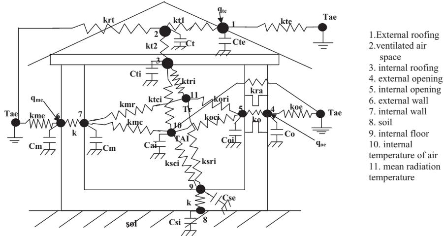
**Fig. 1.** Thermal node model of house and its electrical analogy.
