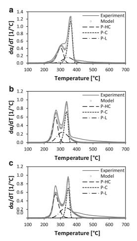
Fig. 7 Comparison between experimental and modeled decomposition curves of **a** BG at 10 °C/min, **b** CS at 10 °C/min, and **c** OPS at 10 °C/min. Modeled curves generated using the calculated *Ea* and *A* values presented in Table 7 for biomasses and their pseudo-components
