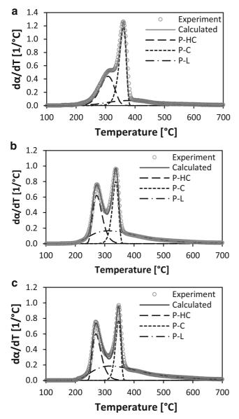
Fig. 3 Comparison between experimental curves and Fraser-Suzuki deconvolution results of a BG at 10 °C/min, b CS at 10 °C/min, and c OPS at 10 °C/min. P-HC pseudo-hemicellulose, P-C pseudo-cellulose, P-L pseudo-lignin
