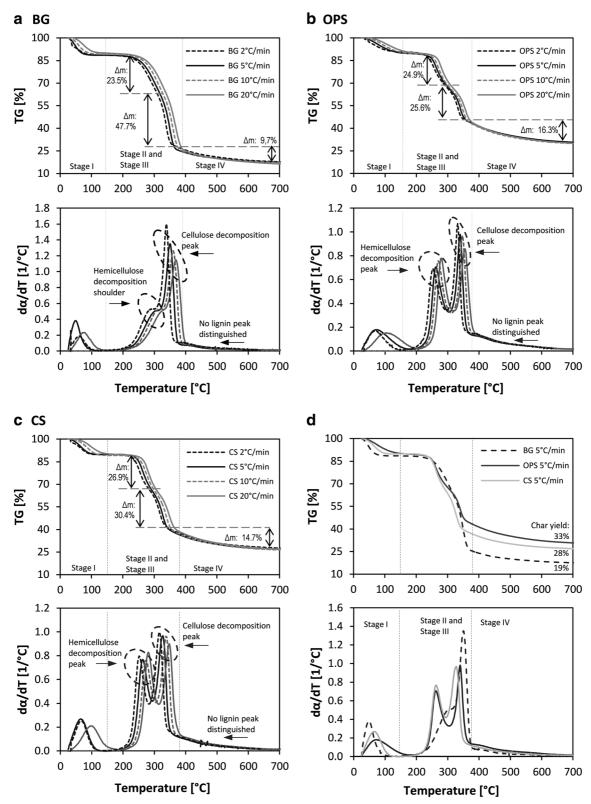
Fig. 2 TG and DTG curves at 2, 5, 10, and 20 °C/min. a *Guadua angustifolia* Bamboo guadua (BG). b Oil palm shells (OPS). c Coconut shells (CS). d Comparison of TG and DTG curves at 5 °C/min. Mass loss values and char yield are presented in a dry basis
