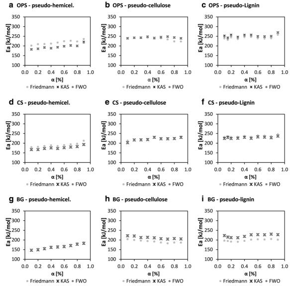
Fig. 4 Apparent activation energy values of BG, CS and OPS pseudo-components, as a function of reaction extent
