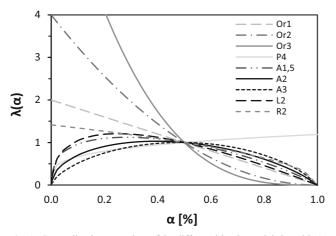
Fig. 1 Generalized master plots of the different kinetic models in Table 2, constructed according to Eq. 6
