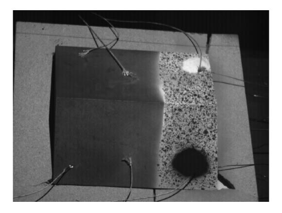
Fig. 14. The right side of the mould was painted for the second experiment in order that the displacement/strain fields could be obtained. each point of its surface are obtained:
