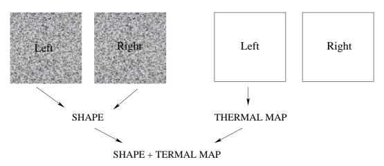
Fig. 11. Shape/Temperature measurement using the same sensor.
