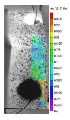
Fig. 19. The area that has been used to analyze the strain field.
