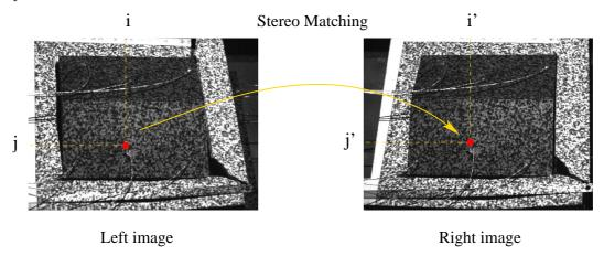
Fig. 10. A correlation-based image matching algorithm was used to find the stereo-corresponding pixels within a given stereo pair of images.
