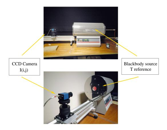
Fig. 3. Our radiometric calibration setup. many processes involving high temperature measurements.
