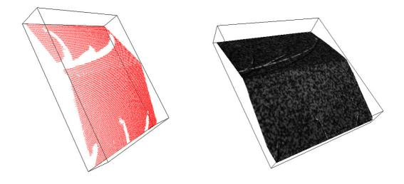
Fig. 12. 3-D shape of the mould obtained by stereo-correlation ; (left) the cloud of3-D points and (right) the image texture overlaid onto the 3-D shape.
