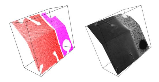
Fig. 16. 3-D shape of the mould obtained by stereo-correlation. (left) the cloud of 3-D points and (right) the image texture overlaid onto the 3-D shape.
