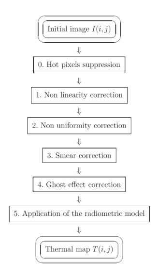
Fig. 2. Summary of the CCD camera corrections for thermal measurements. If the non linearity and non uniformity are not corrected, this can affect the difference of temperature between two adjacent points, which can be a serious problem to compute thermal gradients [22].
