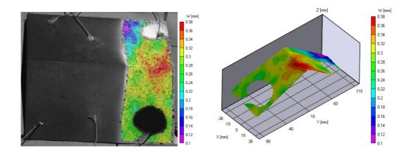
Fig. 17. Any computed value (here the W out-of-plane displacement value) can be overlaid onto the image (left) or onto the 3-D shape (right).
