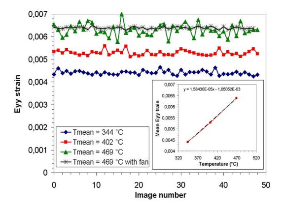
Fig. 20. Strain analysis: from the mean  $\varepsilon_{yy}$  strain evolution over the sequence of 50 images acquired at each level of temperature loading it can be seen that very much more stable strain values are obtained when a fan is used. Estimation of the coefficient of thermal expansion (CTE) of the material from the mean strain values computed at 3 temperature levels (mean temperature given by the thermocouples).
