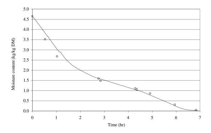
Figure 6 – Drying rate curve (sludge A,  $T_{reg}\!=180^{\circ}\text{C},\,m_{ini}\!=3.5~kg$  )
