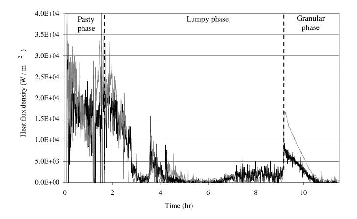
Figure 5 – Comparison between the measured and computed drying kinetics in the batch agitated dryer (sludge A,  $T_{reg}$  = 180°C,  $m_{ini}$  = 3.5 kg )
