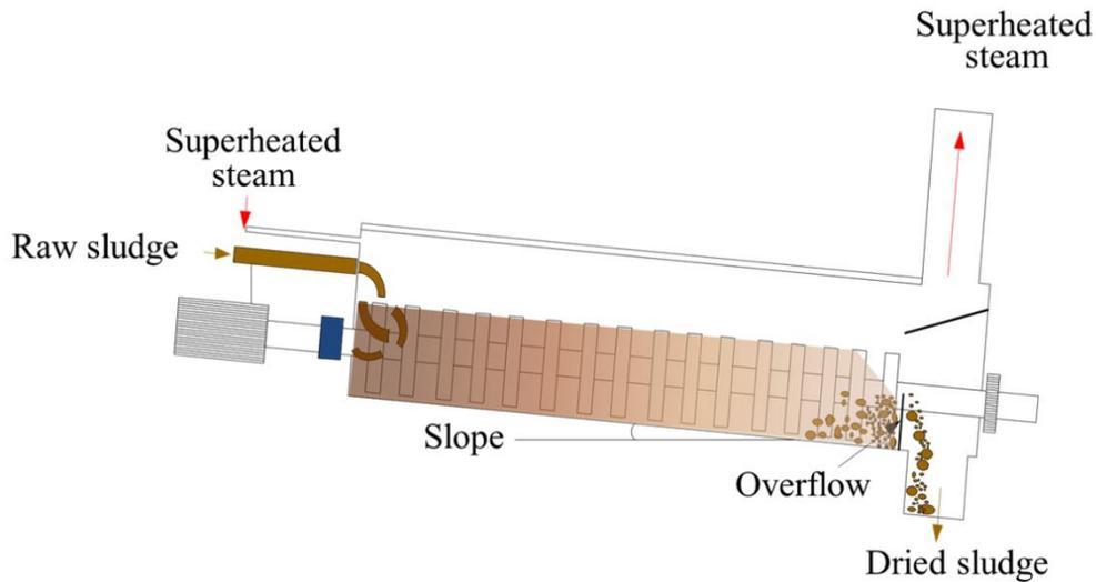
*Figure 1: Scheme of the continuous paddle dryer*
