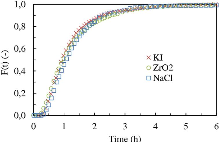
Figure 6: Cumulative RTD obtained for three successive injections of different tracers during a single experiment
